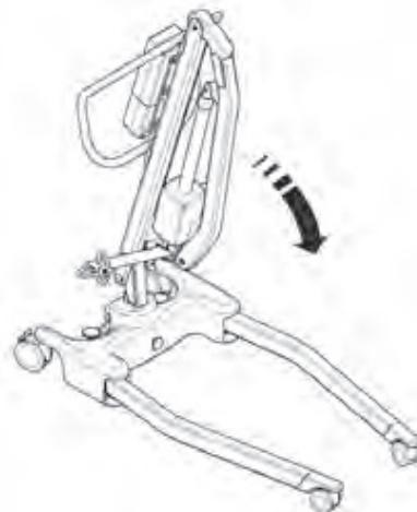
4. Lift the folded Advance upright (using the legs and push handle as a guide) being careful that the mast and boom stay together as you tilt upright.
