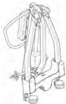
2. Release the leg and mast assembly by unfastening the restraining strap from the wheels. This strap will retract neatly into the top of the mast section.
