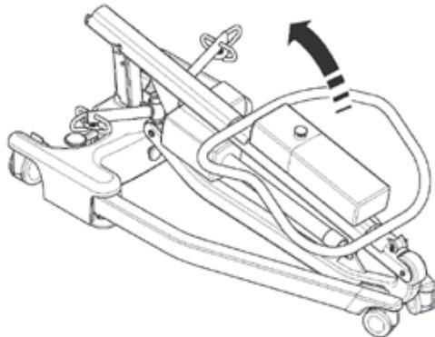
4. Lift the mast assembly upright (using the top of the push handle), and drop the mast into the slot (1), tighten mast lock knobs (2), release braked castors (3).
