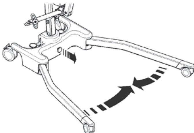
3. Loosen the mast locking device sufficiently to allow the mast to be lifted upwards. Lift the mast fully until the upper stop is reached. Carefully fold the mast towards the legs. Use the push handle to assist this action.
